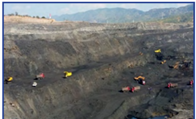
▪ High walls & closely dumped waste materials at Izuma B (left) in comparison to modern best-mining practices currently in place (right)
