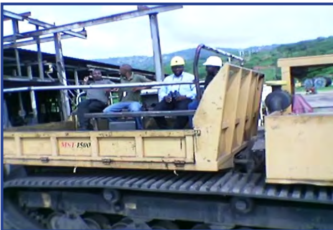
▪ In absence of 4x4 vehicles - tracked man-carrier (MOROOKA) used to navigate the hostile terrain
