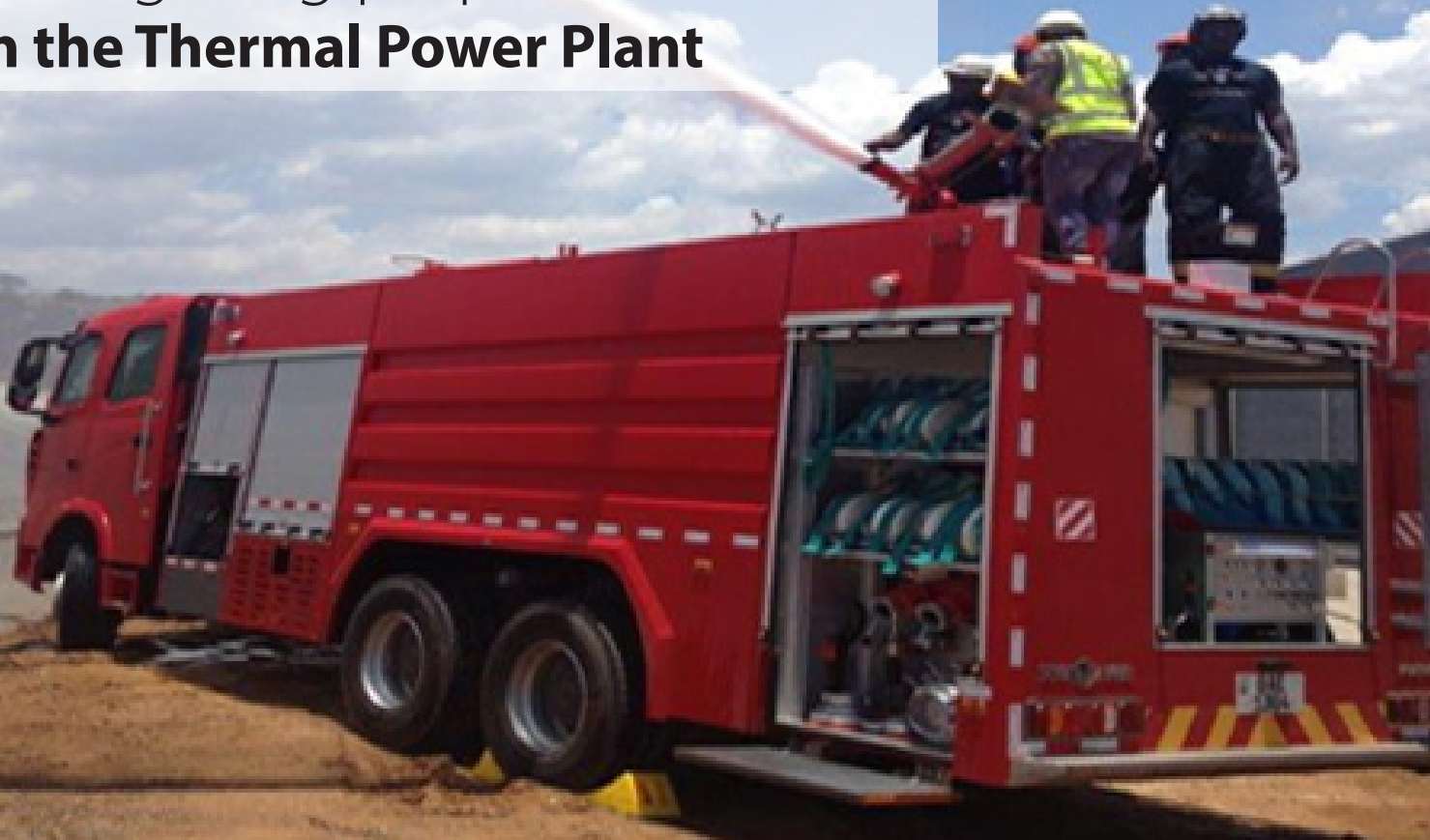
■ Figure 1 Newly procured Fire Tender. MCL recently acquired a - SINOTRUK Firefighting engine with 10,000L Water tank and 1,000L Foam tank
